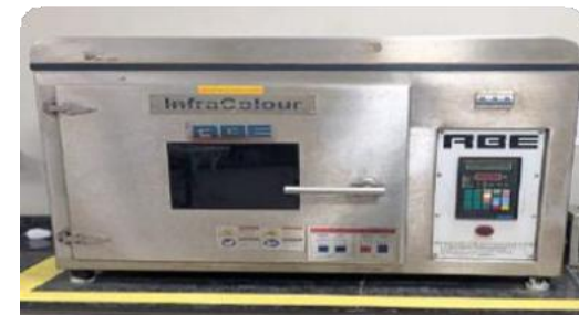
IR Dyeing Machine For Lab Batch Dyeing In Application Lab
