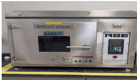
IR Dyeing Machine for Lab batch dyeing in Application Lab
